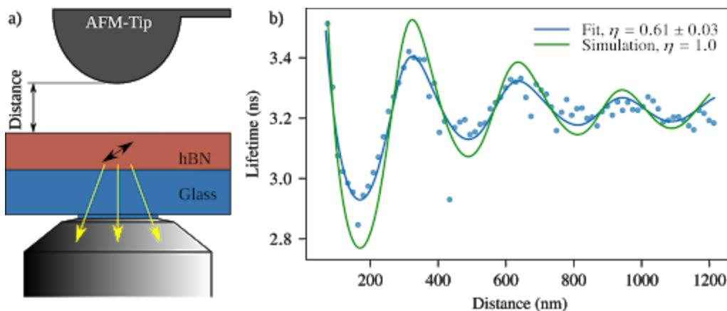
*Schematics of the performed experiment and a distance dependent lifetime measurement.*
